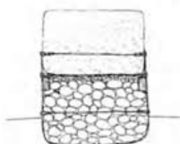
Rock-Filled Gabion Basket
